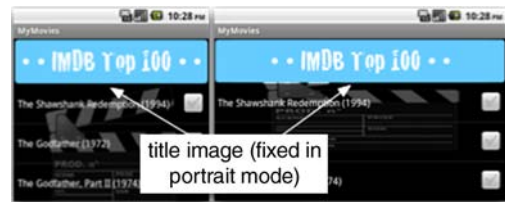
Figure 4.15 The title image now scales correctly in landscape mode. This is achieved by stretching only those parts of the image that are safe to stretch (they don't result in distorted imagery), as defined by the nine-patch format.
