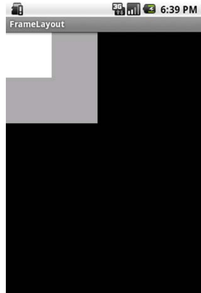
Figure 4.4 Two views arranged using FrameLayout . Note how one view lays on top of the other and both are pinned to the top-left corner.
