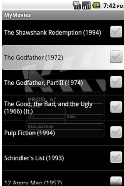
Figure 4.10 The list view selector using a custom shape drawable. Note how we used a custom gradient that goes across the selector horizontally.
