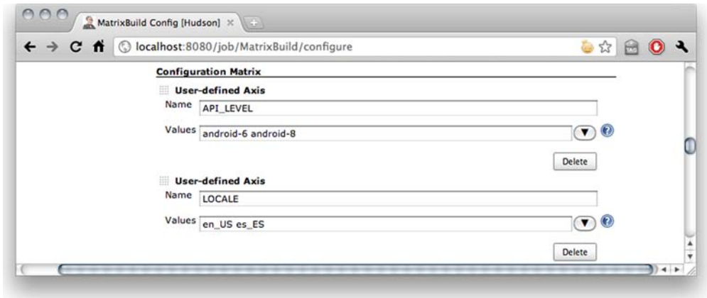
Figure 14.18 The configuration matrix defines the axes and the values each axis can take. For our example, we have an API level (platform version) and language axis. Values for each axis are entered directly, separated by a blank.
