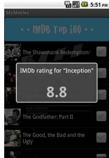
Figure 9.6 Long pressing any of the movie list elements will dispatch a call to the TMDb movie web service and retrieve information about that movie. From that information, we show the official IMDb rating in a pop-up dialog.
