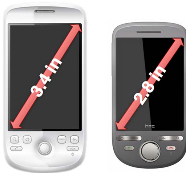
Figure 4.16 Different Android devices may come with different display configurations. Whereas the HTC Magic (left) comes with a 320x480px (160dpi) 3.4 inch screen, the HTC Tattoo has a smaller, lower-resolution 240x320px (120dpi) 2.8 inch screen.
