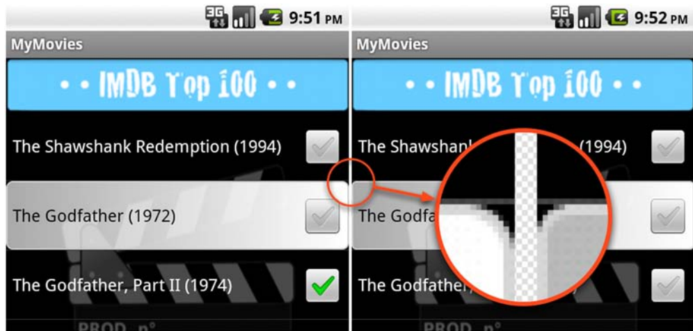
Figure 4.20 Corner radii mismatch on a high-density screen. On the left side, the radius was specified using density-independent pixels (dip), where the right side uses absolute pixels (px), resulting in a physically smaller corner radius.
