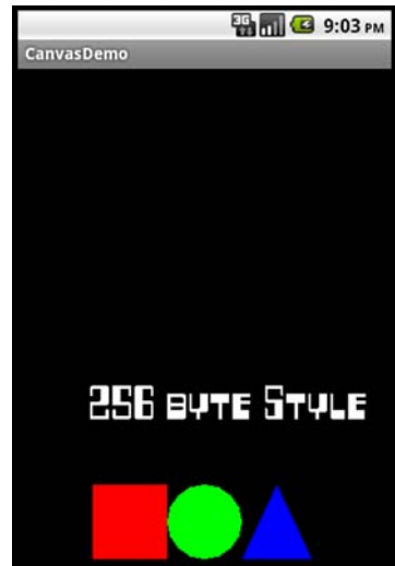
Figure 12.6 Drawing text on a Canvas using a true type font
