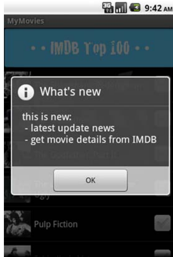
Figure 9.2 On every application start, we show a message dialog to the user with the latest update notes. The text in the dialog is fetched from a web server instead of being bundled with the APK.
